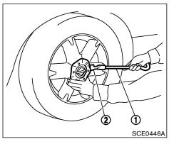
Removing wheel cap (if so equipped)
