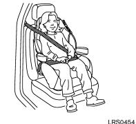
5. Pull the shoulder belt portion of the seat belt toward the retractor to take up extra slack. Be sure the shoulder belt is positioned across the top, middle portion of the child's shoulder. Be sure to follow the booster seat manufacturer's instructions for adjusting the belt routing.
