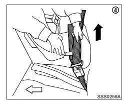
4. Allow the belt to retract. Pull up on the belt to remove any slack in the belt.
