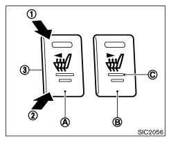
The front seats are warmed by built-in heaters. The switches located on the center console can be operated independently (driver side seat ( $\mathbf{A}$ ) and front passenger side seat ( $\mathbf{B}$ )) of each other.
