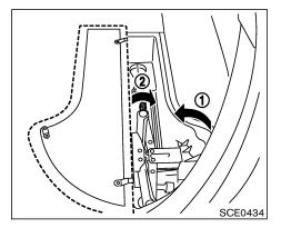
Pull up the floor cover (1) as illustrated and remove (2) the jack and tools.
