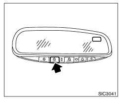
Using both hands, simultaneously push and hold both the HomeLink<sup>®</sup> button you want to program and the hand-held transmitter button.
