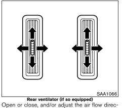
Open or close, and/or adjust the air flow direction of ventilators.
