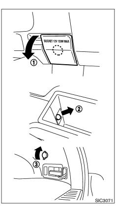
The power outlet is for powering electrical accessories such as cellular telephones.
