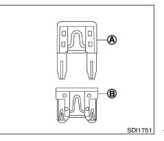
Some vehicles are equipped with engine compartment and passenger compartment fuse boxes that use only type (A) fuses. Other vehicles are equipped with type (A) fuses in the engine compartment fuse box and type (B) fuses in the passenger compartment fuse box.
