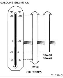
SAE 5W-30 viscosity oil is preferred for all ambient temperatures. SAE 10W-30, 10W-40 viscosity oil may be used if the ambient temperature is above  $0^{\circ}F(-18^{\circ}C)$ .
