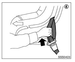
4. Allow the belt to retract. Pull up on the shoulder belt to remove any slack in the belt.
