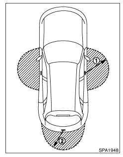
Operating range of the door lock/ unlock function
