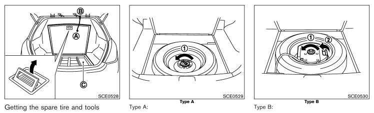
Pull up the floor cover and hang the strap (A) to upper body (B) as illustrated. Remove the under tray (C) (if so equipped).
