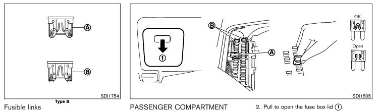
If any electrical equipment does not operate and fuses are in good condition, check the fusible links. If any of these fusible links are melted, replace only with genuine NISSAN parts. Never use a fuse of a higher or lower amperage rating than that specified on the fuse box cover. This could damage the electrical system or cause a fire.
