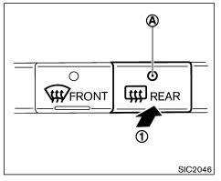
To defog/defrost the rear window glass and outside mirrors (if so equipped), start the engine and push the switch on (1). The indicator light (A) will come on. Push the switch again to turn the defroster off.
