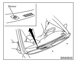
The sensor on the instrument panel helps maintain a constant temperature; do not put anything on or around this sensor.
