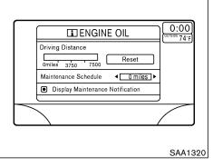
To set the maintenance interval, select the "Maintenance Schedule" key by using the joystick and move the joystick to the right or left.
