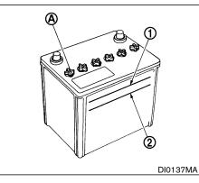
Check the fluid level in each cell. It should be between the UPPER LEVEL (1) and LOWER LEVEL (2) lines.
