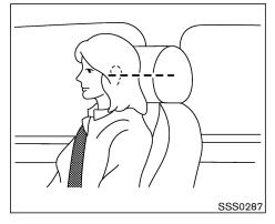
Adjust the head restraints as illustrated so the center is level with the center of your ears.
