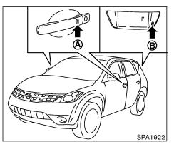
When you carry the Intelligent Key with you, you can lock or unlock all doors by pushing the door handle request switch (A) or lift gate request switch (B) within the range of operation.
