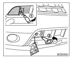
VEHICLE RECOVERY (Freeing a stuck vehicle)
