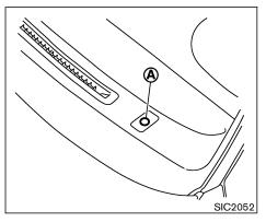
Be sure not to put anything on top of the photo sensor (A) located on the top lefthand side of the instrument panel. The photo sensor controls the autolight; if it is covered, the photo sensor reacts as if it is dark and the headlights will illuminate.
