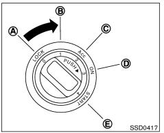
The ignition lock is designed so that the ignition switch cannot be turned to LOCK and removed until the selector lever is moved to the P (Park) position.
