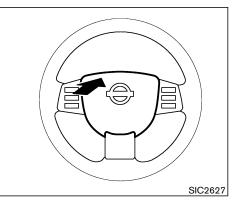
To sound the horn, push the center pad upper area of the steering wheel.
