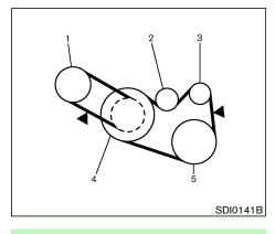
Visually inspect each belt for signs of unusual wear, cuts, fraying, oil adhesion or looseness. If the belt is in poor condition or loose, have it replaced or adjusted by a NISSAN dealer.
