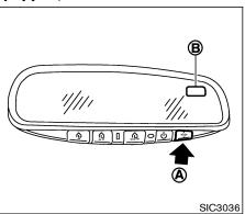
When the compass switch (A) is pushed, the compass display (B) will indicate the direction the vehicle is heading.
