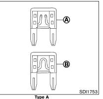
If any electrical equipment does not operate, check for an open fuse.
