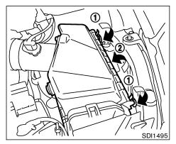
To remove the filter from the air cleaner, push down the lock pins 1 and pull the unit upward 2.
